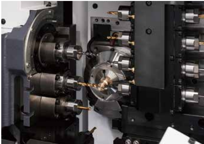
Simultaneous machining with two tools on the front face
