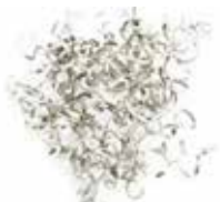
Chips generated by conventional cutting
