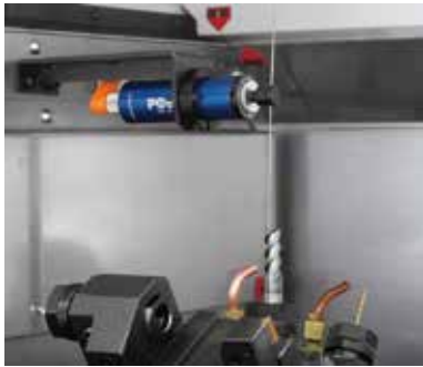
Drill breakage detector Drill breakage is detected by the swing cylinder. The machine stops when breakage is detected, and a second accident can be prevented.
