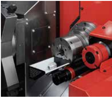
Part catcher These optional devices are indispensable for bar work.
