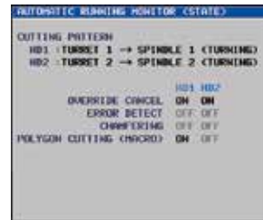
Automatic running monitor (status)
