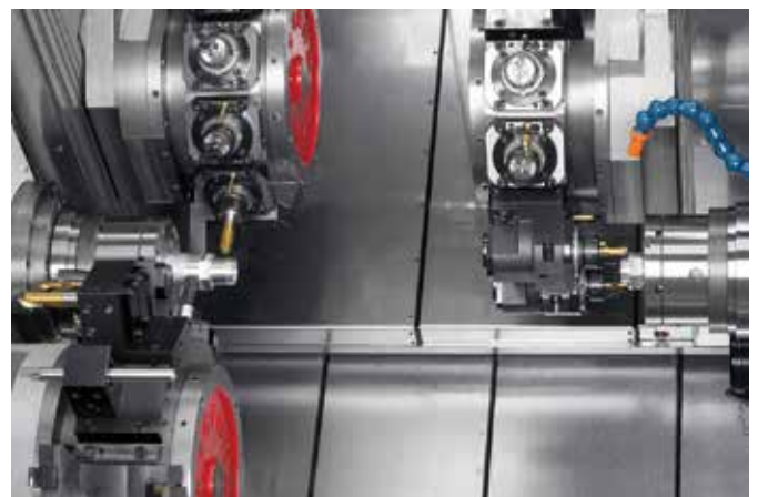
Simultaneous complex machining with three turrets
