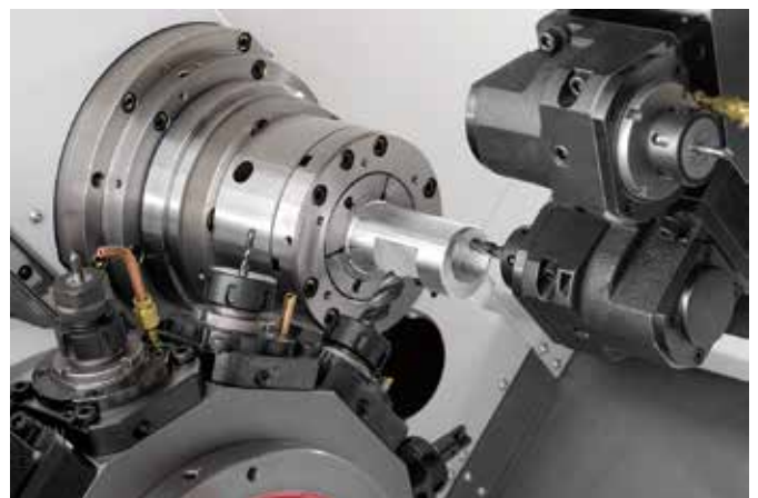
Simultaneous complex machining with two turrets
